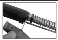
11) Remove the barrel nut locking screw. Note: There are two threaded holes on the barrel nut but only one set screw is used for purposes of locking the nut in the clocked position.
