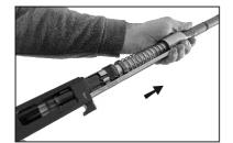
13) Remove the barrel from the receiver
