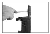
7) Using a hex/Allen wrench, remove the bolt that holds the upper and lower together.
