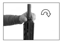
2) Using the provided spanner wrench loosen and remove the castle nut that holds the handguard in place in the clockwise direction.
