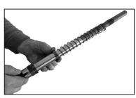
**15)** Slide off barrel nut, escutcheon and recoil spring.
