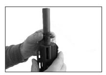
**3)** Remove the O ring if it does not remain in the groove of the handguard nut.
