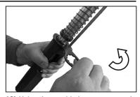
**12)** Using the provided spanner wrench, remove the barrel locking nut in the counter clockwise direction.
