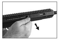
**4)** Pull out the charging handle by firmly holding on to it.
