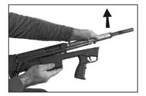
8) By pulling the lower receiver back push and lift on the upper receiver to separate the two.
