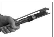
**14)** Push bolt carrier toward the barrel hood compressing the recoil spring. Swing the bolt carrier away from the barrel hood and remove the bolt. Everything will be free at this point.
