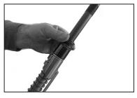
9) Remove the gas system locking nut in the clockwise direction.
