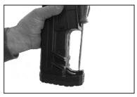
**6)** Remove the Philips screw that holds the back stock pad in place.
