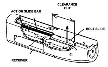
Fig. 10 - Bolt slide installation/removal
