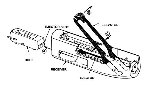
Fig. 11 -- Elevator removal
