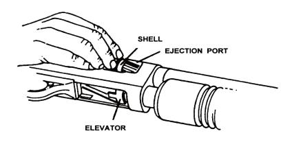
Fig. 5 -- Loading through the ejection port
