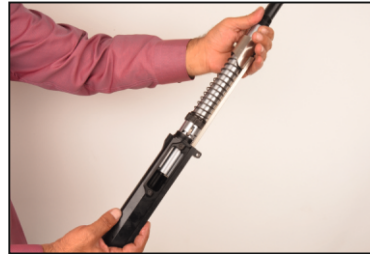
11) Separate the Barrel from the Upper Receiver
