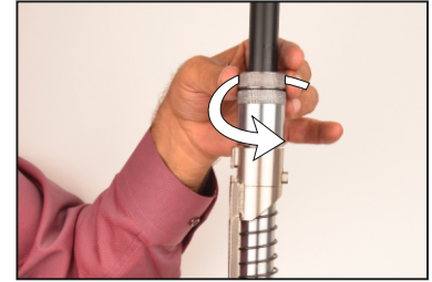
9) Take out the Gas Block Adjust Screw by turning counterclockwise and take out the Gas Block by turning clockwise
