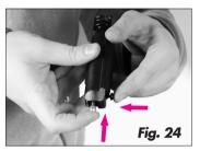
which retains it in the bolt. Push the cross pin in fully against the side of the bolt. The resistance of the "O" ring is designed to prevent the pin from working loose during normal operation (fig.24)
