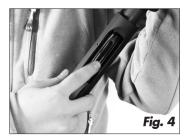
the operation until the magazine is completely loaded. The 12 gauge magazine can hold four 3" (76mm) or 2<sup>3/4"</sup> (70mm) cartridges. To comply with federal and or local laws and regulations currently in effect, the P3000 comes with a limiter plug installed which reduces the magazine capacity to two rounds.
