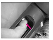
carrier downward, push the front end of the shell latch in with your right hand index finger (fig. 14)
