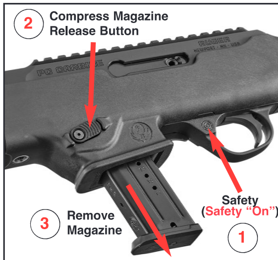
Figure 19. If the hammer is cocked, the safety should be “ON” when the magazine is being removed or inserted. When the magazine release button is pushed in, the magazine is released. Depress the button with your thumb and at the same time grasp the magazine and draw it downward out of the firearm. REMEMBER to check to be sure the chamber is empty after removing the magazine!
