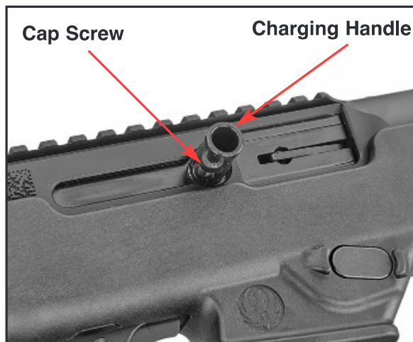
Figure 16. Loosen & Remove Charging Handle Screw
