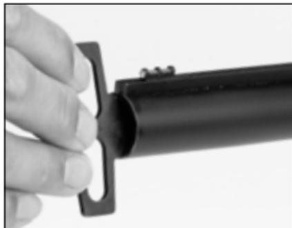
**Use the choke tube wrench to remove and install choke tubes.**
