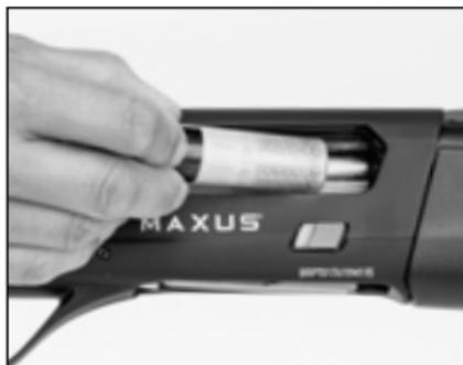
Insert a shell through the ejection port into the breech.
