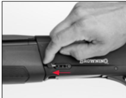
**Push the Magazine Cut-Off forward to unblock the magazine.**
