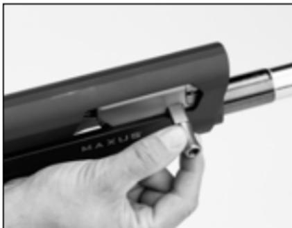
Pull outward to remove the bolt handle.
