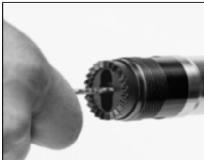
Use a key or screwdriver to press in on the three-shot adaptor, then rotate a quarter-turn.
