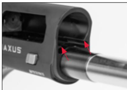
Lightly lubricate the bolt rails inside the receiver.
