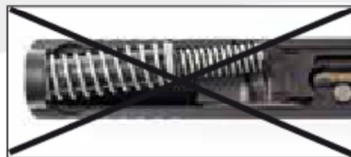
5.1.2 Fig. 3: Spring misaligned
