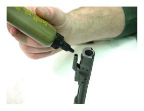
15. Dry the key of the bolt carrier assembly with a pipe cleaner. Place one drop of lubricant inside the key.
