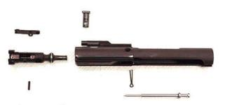
1. Clean all parts and outer surfaces of the bolt carrier assembly with a swab saturated with cleaning solvent.
