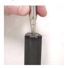
Remove the spring and attached follower from the magazine shell. The spring will exit the shell easily, but the follower must be twisted and withdrawn, rear first. Do not remove the spring from the follower.
