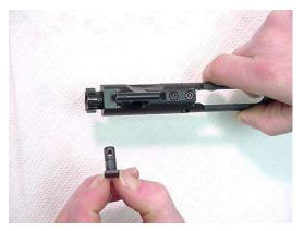
7. Give the bolt cam pin a ¼ turn and lift it out.
