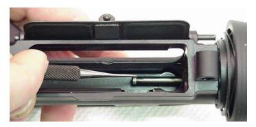
3. Use a worn out bore brush to clean the outside surface of the protruding gas tube (U-9) (get the sides and bottom from the bottom of the upper receiver). This procedure ruins the brush.
