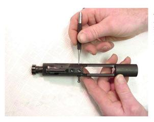
4. Move the bolt assembly forward to the unlocked position and remove the firing pin retaining pin. Do not open or close the split end of the firing pin retaining pin.
