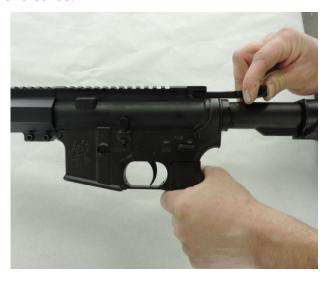
2. Push upward on the magazine until the magazine catch engages and holds the magazine. Pull down on the magazine slightly to make sure that it is locked in place.
