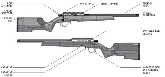
Your safety lever is located to the right of the bolt shroud (right handed rifles). The safety mechanism provides some degree of protection from accidental or unintentional discharge under normal usage when properly engaged and in good working condition.
