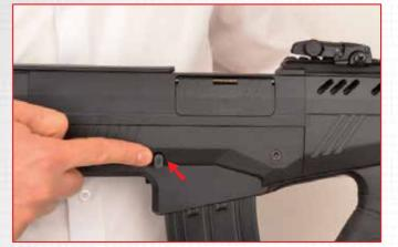
**1.** Remove the magazine by pushing the release button.
