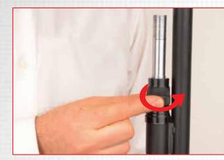
7. Remove the barrel cap by unscrewing it.
