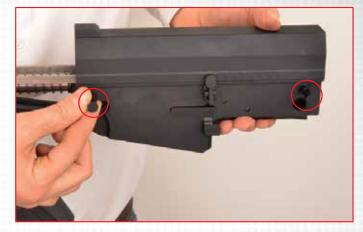
**15.** Push the pins in the front and the back, and pull them from the other side until they unlock.
