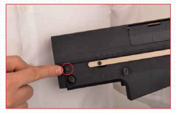
**14.** The pins are used to seperate the upper from the trigger housing.
