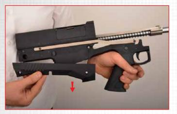
**13.** Remove the the covers located on both sides carefully.
