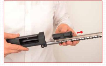
**17.** Pull the bolt assembly in arrow direction and remove it carefully.
