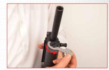
**3.** Use the tool to remove the cover in the front.
