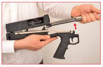
**16.** Slightly push the bolt assembly backwards until it unlocks. Then seperate the trigger housing from the upper by pulling in arrow direction.
