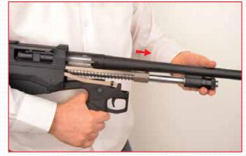
**8.** Hold the pilstol grip and push the barrel in arrow direction.
