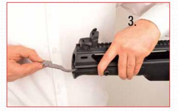
**5.** Hold the charging handle tight and remove the cover in the front with a tool.
