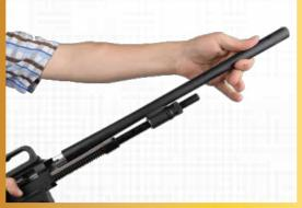
4. Pull the bolt to the rear slightly and remove the barrel as you are letting the bolt slide forwards. Slowly release the bolt to clear the recoil spring/bolt carrier as the barrel comes out.
