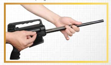
5. Turn the ratchet downward to release the carrier.
