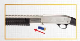
With trigger locked, insert shell upward into bottom of receiver and push forward into magazine tube past cartridge stops. Repeat until magazine tube is full.
