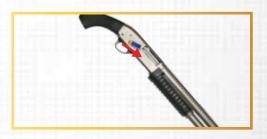
Turn gun over, trigger guard up, and barrel pointing down. Press cartridge stop left to release shell from magazine. Remove shell and repeat until magazine is empty.
