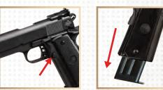
To unload, press the magazine release and remove the magazine. If the slide is in the forward position, pull it to the rear and retain by pushing the slide stop up. Inspect the chamber to make sure that the pistol is clear and unloaded. If there is a shell or unfired cartridge in the chamber, manually remove it before pressing the slide stop down. Your gun is now unloaded.
