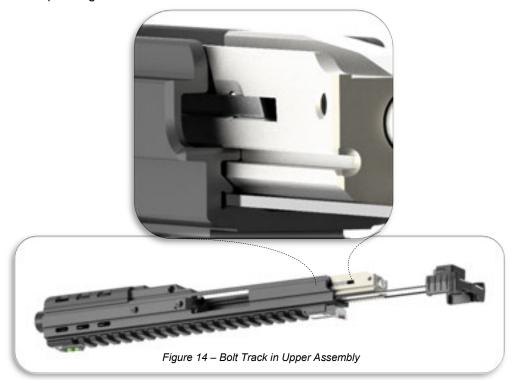
6. Push the buffer forward a little while holding the operating handle before the buffer goes into the upper so that the slots in the buffer align with the rails in the upper.
