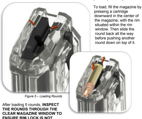
**OCCURING** (Figure 5). The first two rounds to be loaded should be pushed to the outside of the magazine, and the other rounds above it should stagger evenly. Also verify that the rim of each round is in front of the rim of the round directly below it. If a round is not in the correct place, you can use the windows on the side to correct the placement, and then tap the side of the magazine onto a table or similar hard object to re-seat the rounds.
