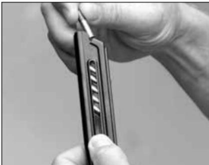
Depress the magazine's follower button with the thumb of one hand while inserting cartridges with the other hand.
