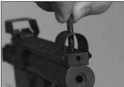
**With the sight adjusting wrench, rotate the blade to the desired width.**
