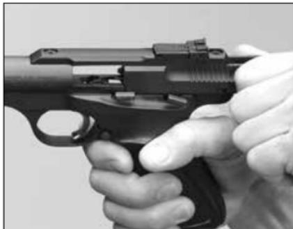
**Release the slide to feed the first cartridge from the magazine into the chamber.**
