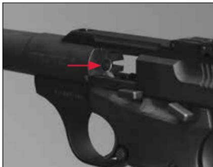
**With the slide locked to the rear, inspect the chamber to be sure it is empty.**
