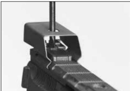
**To adjust elevation, turn the elevation screw located just forward of the rear sight notch.**
