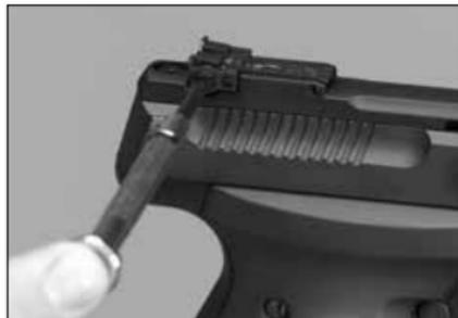
To adjust windage, turn the screw located on the right side of the sight.
