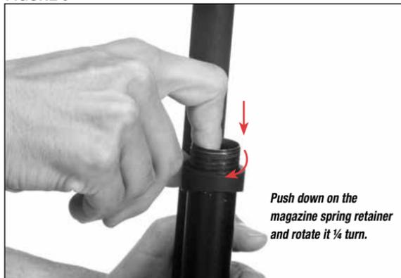
2. The magazine three-shot adaptor is located underneath the magazine spring retainer and is under pressure from the magazine spring. Using your index finger or a large blade-type screwdriver, press the magazine spring retainer into the magazine approximately 1" and rotate it  $\frac{1}{4}$  turn (Figure 9, page 16).
