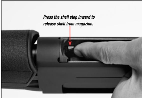
stop, located on the inside-right of the ejection port, to release a shell from the magazine (Figure 12, page 21). Press the shell stop again to release the next shell.
