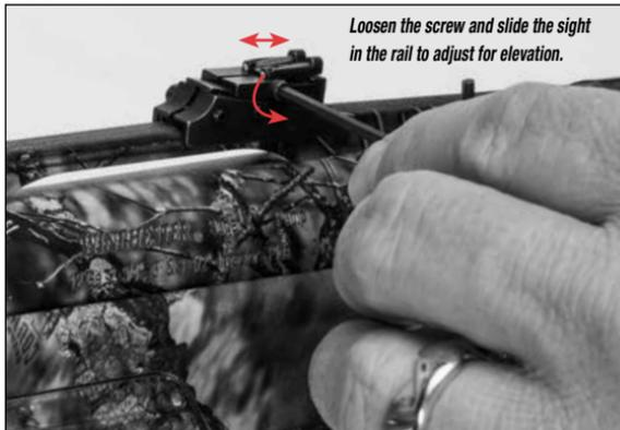
4. Tighten the screw on the top of the sight. Do not overtighten.
