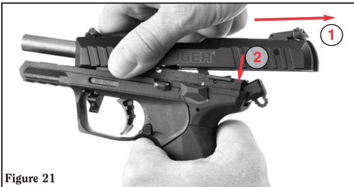
Note that light downward pressure will be required to depress the hammer slightly so that the slide can engage the frame rails. (See Figure 22.)
