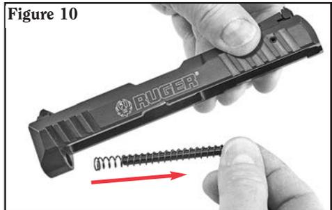
8. This completes normal field stripping for routine cleaning and lubrication purposes. (See Figure 11.) Further disassembly of the slide or frame components is not recommended and should only be undertaken by the factory.
