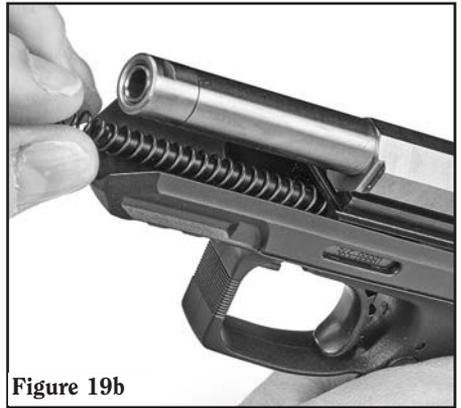
7. Line the recoil spring up with the hole in the chin of the slide. (See Figure 20.)
