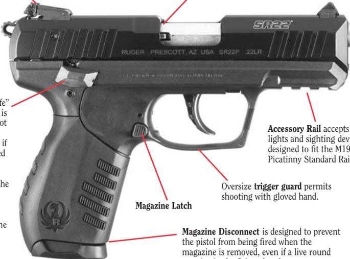
When ambidextrous **manual safety** is in "safe" position, the firing pin is blocked so that it cannot make contact with the cartridge. Additionally, if the hammer is decocked using the safety, the hammer is held away from the firing pin. If the decock is not used, the hammer can be thumb cocked slightly so that the hammer rests on the decock hammer stop.
