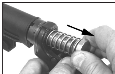
Fig. 95 – Removing non-HK Buffer and Action (Recoil) Spring
