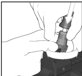
Fig. 7 – Rear Sight Adjustment
