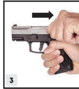
3. Hold the pistol with one hand keeping your finger away from the trigger insert and on the **memory pad**. With the other hand pull the **slide** to its limit and release it, so **slide** will go forward under **recoil spring** pressure and will insert one cartridge in the **chamber**.
