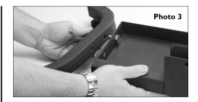
the two short M12 Bolts (K) and fasten the Front Tube (A) to the Main Frame Assembly (B). The Front Tube has feet already installed. Ensure that the tube is oriented
