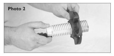
2. Turn the thumbscrew counterclockwise and far enough to install the ram and assembly into the base. Fully install the ram and wheel assembly, allowing the wheel to rest into the base. Secure the ram and wheel assembly into position using the thumbscrew. See **Photo 3**.
