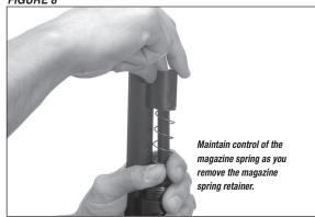
three-shot adapter (plug) and replace the magazine spring retainer.
