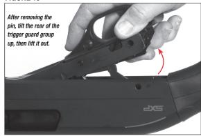
7. With the pin removed, lift the trigger group out of the receiver by lifting upward and pulling rearward (Figure 13).
