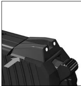
Fig. 7 Rear sight adjustment
