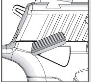
**3. Manual Safety Latch.** By moving the safety fully upward you will block the firing mechanism of the pistol. Keep the safety on while not firing the pistol.
