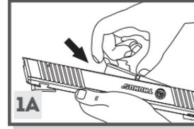
1. Replace the barrel in the slide pushing it to the rearward position (1a). Insert the spring/guide rod sub-assembly into the slide over the barrel (1b).
