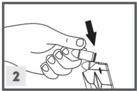
2. To load the magazine, hold the **magazine** with one of your hands and with the other one insert the cartridges one at a time, pressing them down and to the rear. Insert the **magazine** into the pistol until it is held by the **magazine catch**. If the **magazine** is not correctly inserted into the pistol, it can fall out.
