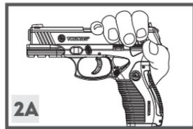
**disassembly latch** down. Push the slide to its forward position before releasing the disassembly latch.
