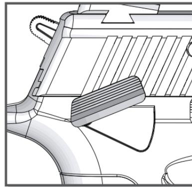
**3. Manual Safety Latch.** By moving the safety fully upward you will block the firing mechanism of the pistol. Keep the safety on while not firing the pistol.
