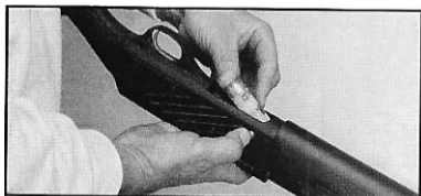
Fig. 7: Turn the shotgun upside down so that the barrel is pointing toward the ground and you are looking at the carrier latch.
