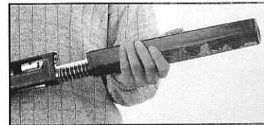
Fig. 2: Remove forend from magazine tube.
