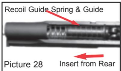
5. Position the arched portion of the recoil spring guide over the barrel directly in front of the barrel link.
