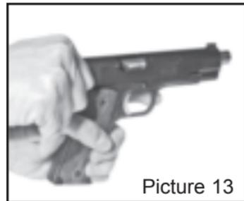
10. Once the slide is in the full rear position, release the slide, letting the slide move freely forward.
