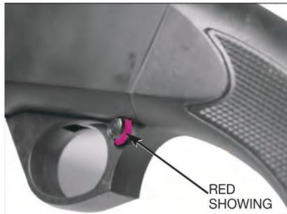
PUSH IN FULLY TO THE LEFT UNTIL BUTTON MOVES NO FURTHER TO BE IN THE “OFF” (FIRE) POSITION.
