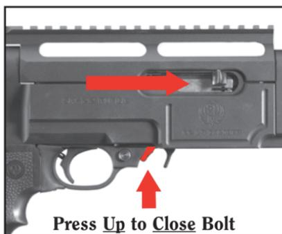
**To release the bolt:** Retract the bolt handle to its extreme rearward position and then press in on the upper section of the bolt lock. Release the bolt and it will move fully forward.
