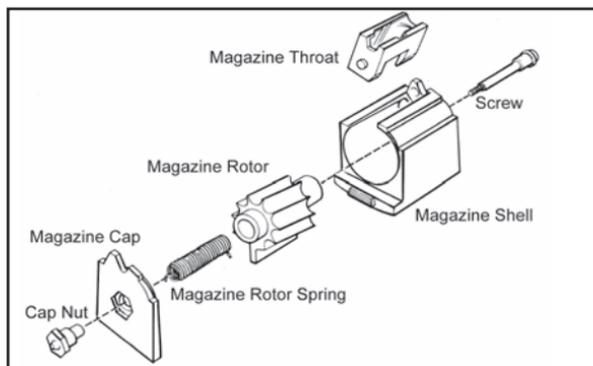
Exploded view of the SR-22 magazine components. This illustration is included to show the relationship and names of the magazine components. As noted in the text above, the magazine should not be disassembled.
