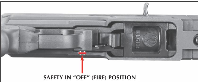
**Figure 3.** The underside of the trigger guard section of the rifle. In this illustration the safety is shown in the “off” (fire) position. The position of the safety and red band indicate the safety is “off.” It should be in this position only when you are actually firing at a target.
