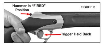
WHEN THE TRIUMPH® IS COCKED AND THE TRIGGER IS PULLED - THE HAMMER CONTACTS THE FIRING PIN (FIGURE 3).
