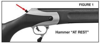
THE HAMMER SHOULD BE IN THE "AT REST" POSITION DURING LOADING AND WHEN CARRYING (FIGURE 1).
