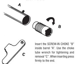
Periodically (each time after 100 shots) remove the SCREW-IN CHOKE and clean internally a and externally using lubricant oil and a piece of flannel cloth.
