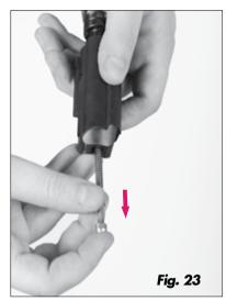
NOTE: Do not disassemble any further as the locking head pin is permanently staked place from the factory.
