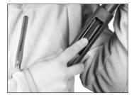
magazine can hold four  $3^{1/2''}$  (89mm) or five  $2^{3/4''}$  (70mm) cartridges. To comply with federal and or local laws and regulations currently in effect, the P3500 comes with a limiter plug installed which reduces the magazine capacity to two rounds.
