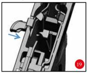
Hook the spring back into the magazine release by reversing the procedure shown in Illustration17.
