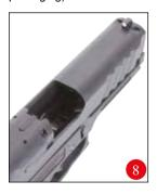
WARNING: Never point a firearm toward anything that it is not safe to shoot. Remove the magazine and lock the slide in the open position before handing the pistol to another person.
