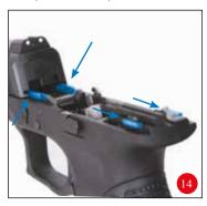
Continue moving the slide onto the frame until the slide is fully rearward. Then, allow the slide to move forward to the closed position. Check that the disassembly latch is in the fully engaged (Illustration 15).
