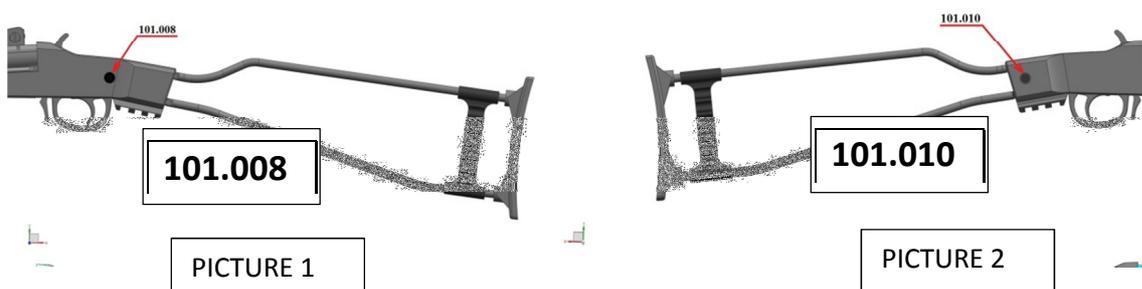
1. Move the stock sideways (right and left) so that it is released and adjust length as desired.
