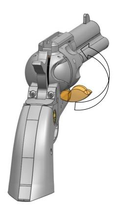
WARNING: Do not carry this revolver with a live round chambered under the hammer and firing pin. Keeping an empty chamber under the hammer is good insurance against accidental firing.
