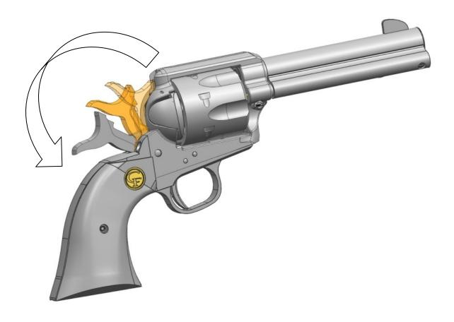
5. Place index finger on trigger, take aim and gently squeeze rearward until hammer is released and falls forward striking the firing pin. Be prepared for loud noise and recoil.
