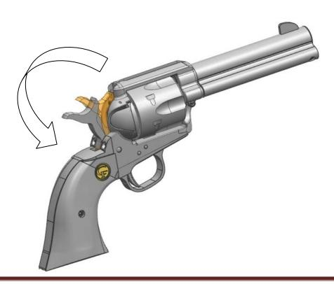
2. open the loading gate (A) on the right rear part of the frame.
