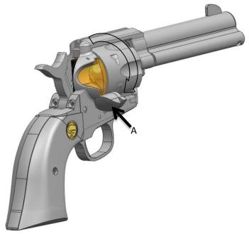
5. Turn cylinder clockwise, by hand, and insert cartridges in chambers until the cylinder is loaded.
