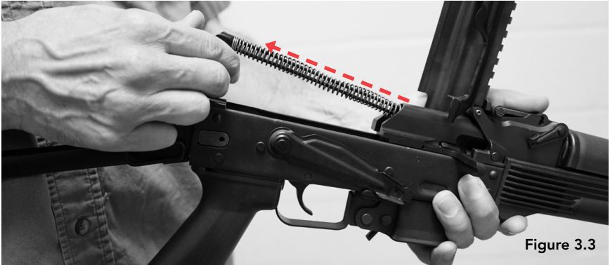
Figure 3.3 — Detaching The Recoil Spring Guide Assembly
