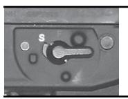
Keep the safety "ON" unless actually firing. Always move the safety to its intended position and check it. The safety is not "ON" unless it is completely "ON." Never depend on a safety mechanism or any other mechanical device to justify careless handling or permitting the rifle to point in an unsafe direction. The only "safe" rifle is one in which the bolt is open, the chamber is empty, and there is no magazine in the gun.
