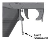
WARNING: Do not manipulate the trigger guard unless the rifle's safety lever is on "S" (SAFE) and unloaded.
