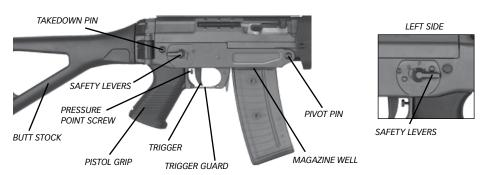
The trigger guard may be released from its normal position to make the trigger accessible for shooting with gloves. For safety reasons the trigger guard must not be released until just before firing the weapon, and after firing should be immediately returned to the normal (closed) position.
