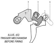
By pulling the trigger (8) and after having overcome the pressure point, the sear (4) releases the hammer (3) which strikes the firing pin (9). The sear (4) falls downwards.
