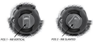
When cycling or ejection problems are encountered due to heavy fouling, the gas valve can be moved to Position 2 by rotating clockwise as far as the stop. In this position, a larger gas volume is released against the operating rod. The need to use the gas valve in Position 2 is an indication that the rifle requires cleaning.
