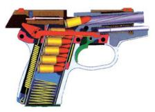
During the complete recoil motion, the hammer is fully disengaged and follows the slide acting like an extra recoil spring. When the trigger is released the trigger bar moves backwards and behind the hammer catch. The pistol is then ready for the next shot.
