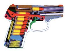
The ignited powder gas drives the bullet forward through the barrel and simultaneously drives the slide and barrel backwards. After about 3/16" (5 mm) the barrel is cammed down by the assembly pin and releases the slide to travel back extracting the case. On it's way back, the slide is gradually slowed down by the recoil springs.
