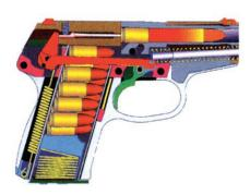
Close to the rear position, the empty case hits the ejector, and is thrown out of the gun. The recoil springs drive the slide forward again. The top cartridge in the magazine is picked up by the breechface and pushed into the barrel. Close to battery the barrel is cammed up positively locking into the slide.
