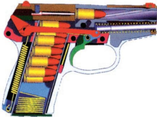
The ignited powder gas drives the bullet forward through the barrel and simultaneously drives the slide and barrel backwards. After about 3/16" (5 mm) the barrel is cammed down by the assembly pin and releases the slide to travel back extracting the case. On it's way back, the slide is gradually slowed down by the recoil springs.
