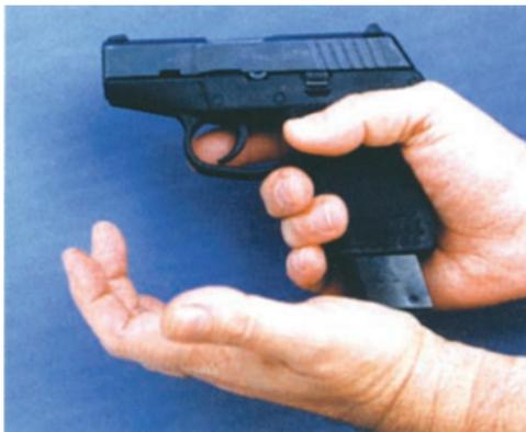
Hold the pistol in one hand with the muzzle pointing in a safe direction and with your finger off the trigger and outside the trigger guard. Insert the loaded magazine into the grip until it is locked in place. Check to assure magazine is secure. Pull the slide back and release. This strips a round from the magazine and seats it in the barrel chamber. At all times keep your hands away from the muzzle.
