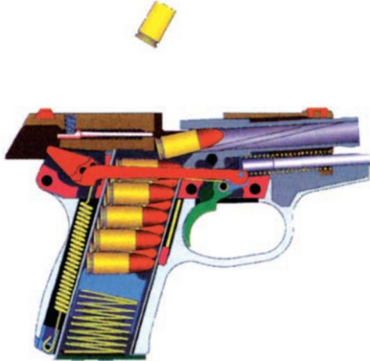
During the complete recoil motion, the hammer is fully disengaged and follows the slide acting like an extra recoil spring. When the trigger is released the trigger bar moves backwards and behind the hammer catch. The pistol is then ready for the next shot.
