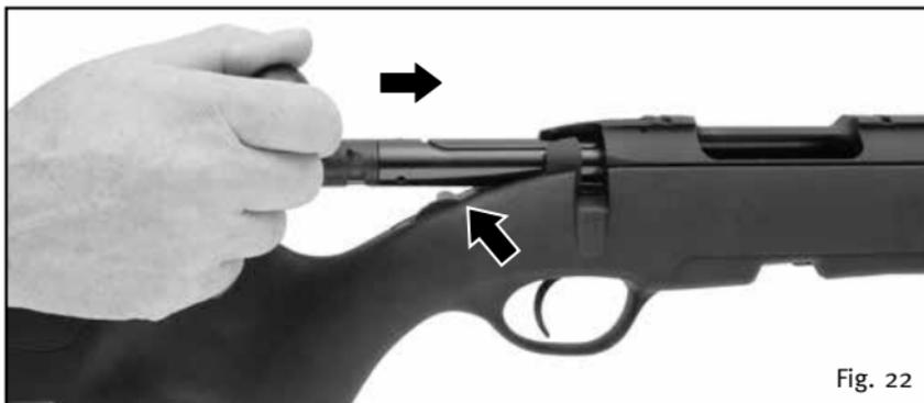
1. First, make certain that the magazine has been removed or locked in second position (Fig. 15) and the weapon is unloaded!
