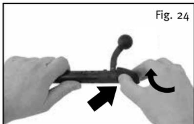
1. Grip the bolt with your left hand. Push in catch lever with your right thumb and simultaneously rotate the bolt sleeve clockwise (arrow shows direction of rotation) until it unlocks with an audible click.
