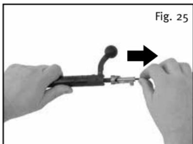
2. Take off bolt sleeve and extract firing pin assembly.
