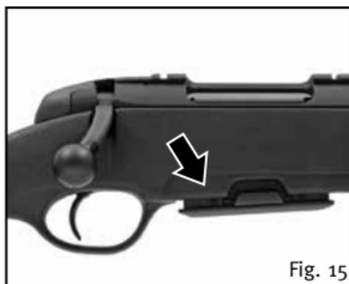
2. Remove magazine or lock it in second position (magazine protrudes by approx. 5 mm/ 0,19").
