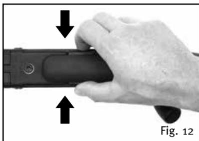
Press the two snap latches at the right and the left of the magazine fully together using thumb and index finger of one hand and remove the magazine while pressing.
