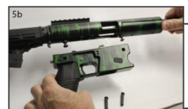
5b. Then pull down the trigger housing to remove.
