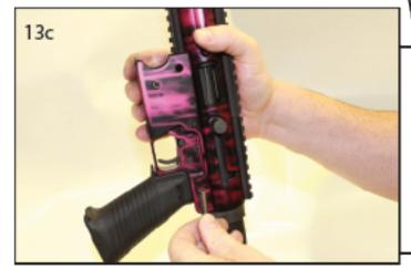
13c. Replace the two receiver cross pins.
