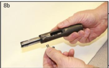
8b. When the firing pin retainer is removed from the bolt, the firing pin and firing pin spring can be removed from the front of the carrier.
