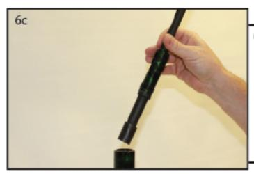
6c. Pull up the barrel to remove completely.
