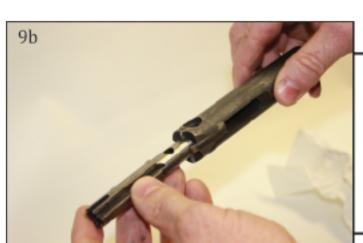
9b. Place the bolt head back into the carrier.
