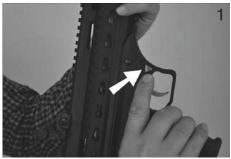
2) Press the release latch magazine to remove it
