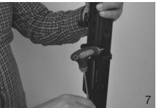
8) Removing the nut seen in the picture unplug the gas chamber and piston
