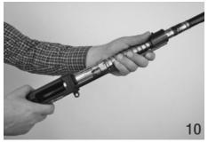
11) Remove the mechanism by pulling the carrier sled back
