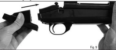
10. Insert Forend Assembly (with barreled action installed) back into corresponding slot rails located in the Thumbhole Stock Assembly. Slide the Forend Assembly back completely until it stops flush against rear Recoil Spring Housing. (Fig. 10)
