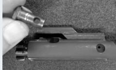
11. Remove the bolt from the bolt carrier body.
