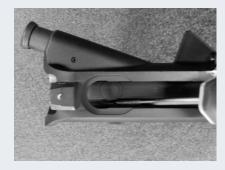
7. To field strip the bolt, make sure that the bolt is in the forward or extended position. Next, remove the firing pin retaining pin. (It looks like a cotter pin and is designed to only go through one side of the bolt carrier.)
