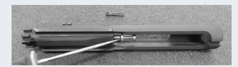
10. Turn the bolt cam pin 90 degrees and remove it from the carrier.
