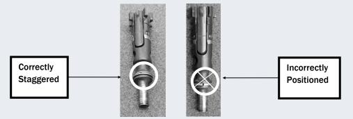
3. Always make sure that the cam pin is installed correctly.
