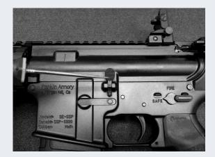
Warning: Do not carry the Pistol with the bolt carrier locked back while a loaded round is in the trough. If the bolt carrier were to get jostled and slide forward, an accidental discharge may result, especially if the safety selector is not set on "Safe."
