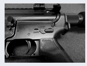
Pull the charging handle all the way back and use the lower portion of the bolt catch to hold the carrier back.
