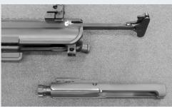
6. Remove the charging handle by sliding the charging handle to the point where the "ears" (or protruding tabs) on the charging handle can slip through the keyway on the upper receiver. When the charging handle is extended out approximately 4.4" from the upper receiver, the ears on the charging handle should be lined up and can slide up through the keyway.
