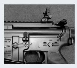
2. Push the charging handle forward until it snaps back into position.
