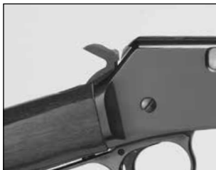
The hammer shown in the half-cock position.
