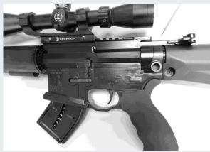
3. Pull the charging handle to the rear, and remove the magazine.
