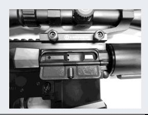
Warning: Never allow a finger to enter the ejection port. If the bolt carrier were to slide forward, it would have considerable force and cause a painful incident!
