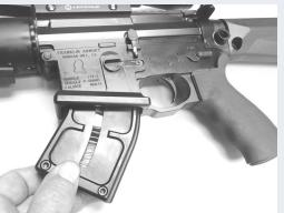
7. Pull the charging handle back all the way, and release it. It is important to allow the charging handle to move forward with full force. Slowing the charging handle down will prevent the carrier from going into battery.
