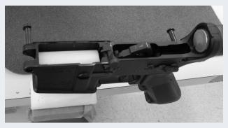
5. Slowly pull the charging handle back and remove the bolt carrier assembly. Be careful not to drop the bolt out as the charging handle comes back.
