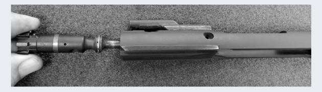
13. Push on the back of the extractor to relieve pressure off of the extractor roll pin. Use an appropriate sized punch to remove the roll pin.
