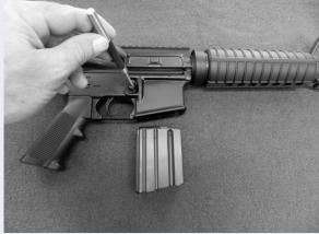
3. Depress the magazine release button and remove the magazine.
