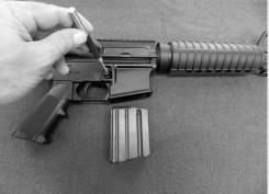
4. Remove the ammunition source by removing the magazine. To do so, depress the magazine release button and pull the magazine out the bottom of the magazine well.
