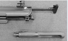
7. Remove the charging handle by sliding the charging handle to the point where the "ears" (or protruding tabs) on the charging handle can slip through the keyway on the upper receiver. When the charging handle is extended out approximately 4.4" from the upper receiver, the ears on the charging handle should be lined up and can slide up through the keyway.
