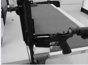
**Warning:** Never dry fire the firearm when the upper and lower are not fully assembled. The steel hammer will hit the rear of the aluminum magazine well and eventually cause it to crack.
