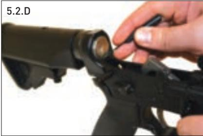
To complete the field strip of the lower receiver assembly, remove the buffer and spring from the buffer tube:
