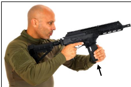
Figure 3-3: Inserting the Magazine
