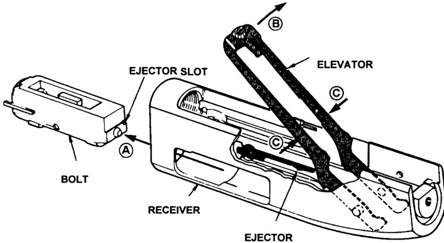
**Fig. 11 – Elevator removal**
